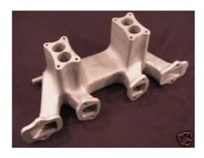
Here above is a vintage racing part for the 254 straight 8 engine a little bit of proof that the 308 was not the only capable engine Hudson had. Matter of fact there was a gallant effort to make the 8 cylinder into a powerhouse like the or rather instead of the 308. Several prototypes were made with full pressure oiling and dual carburetor manifold but the decision was made to build up the 262 to 308 size instead and the rest is history.
